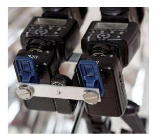
A two-flash adaptation of the single bracket. It has two cross-bars added and uses a standard umbrella swivel.
