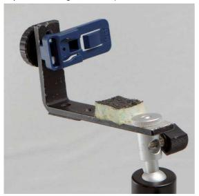
A home-made mount for one or two flashes using a cheap ball swivel, some aluminium bar and a Frio cold shoe. For better security, add a Velcro strap around the head.
